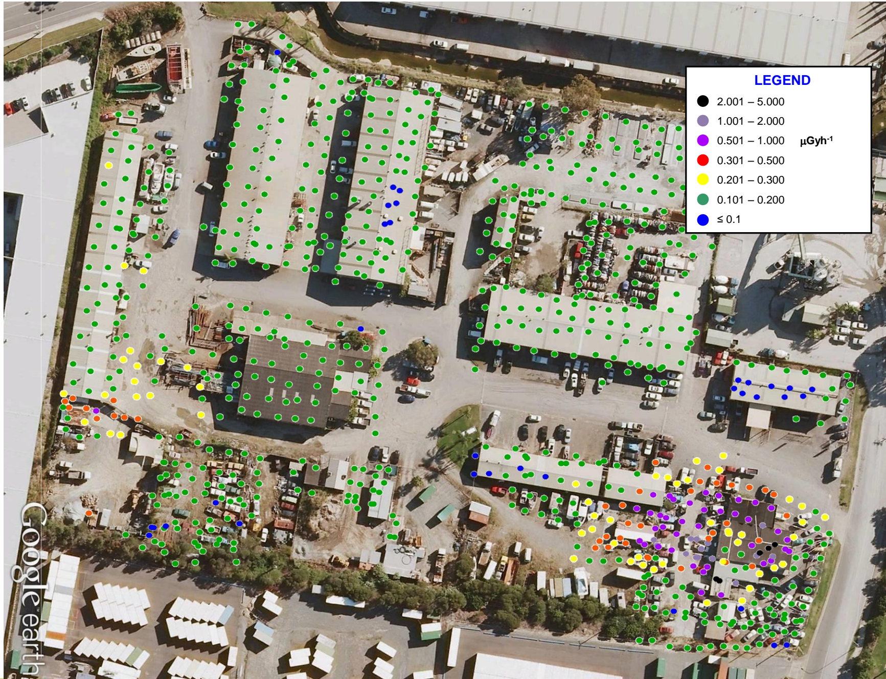
surface gamma radiation survey map of industrial site – abrasive blasting / fill
