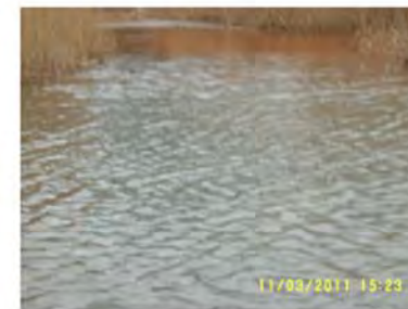
Plate 18 – Rhodamine in reservoir almost two and quarter hours after injection of dye
