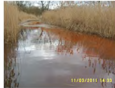
Plate 15 – Rhodamine entering open reservoir (out of the edge of the reed beds), approximately 1.5 hrs after injection
