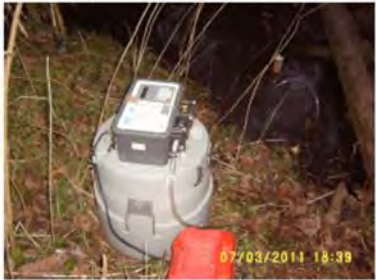
Plate 7 – Autosampler set up at sample location 8 (stream by footbridge)
