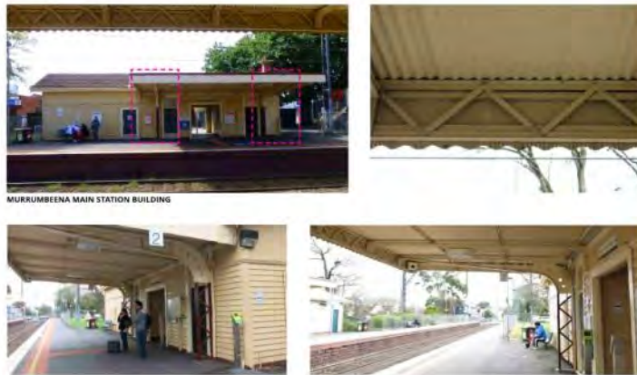
Reuse of Station Canopy Trusses : Preferred option
