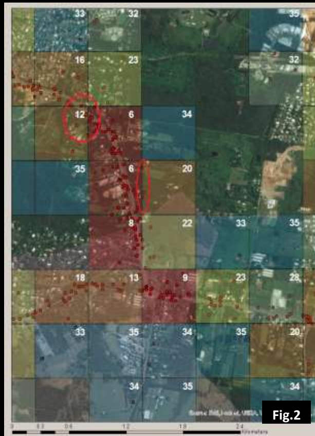
Fig.2. 500m x 500m Grid Overlay method trialled, but some points were split over two cells (circled areas) biasing cell reporting
