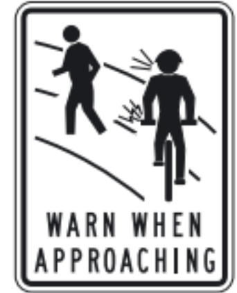
G9-259-2 (b) Warn When Approaching sign encourages path users to call out or use their bells
